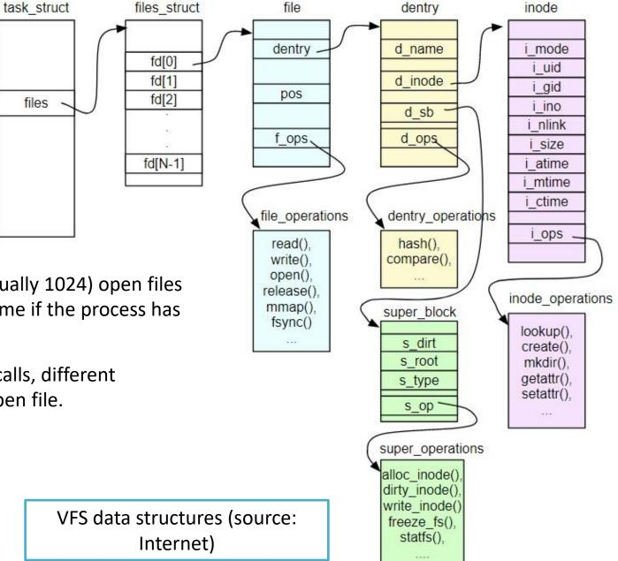
The process can have **NR\_OPEN** (usually 1024) open files (this limit can be **increased** at run time if the process has superuser privileges).
